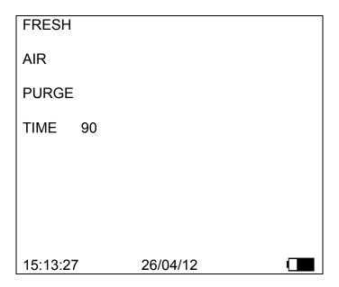
The time will count down in seconds to zero and is pre-set by the analyser. During countdown the analyser will initialise the measuring system, do not block the end of the probe or insert into or near the vehicle exhaust. It also displays some setup values including atmospheric pressure and internal ambient temperature.
