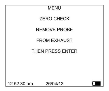
Ensure the probe is removed from the vehicle exhaust and is sampling fresh air, in the garage environment this should be ½ metre or 18 inches above the ground. Once this is done press to activate the pump.
